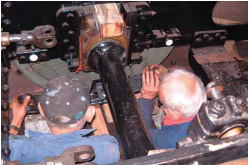
Looking down on Roger and Brian fitting the leaf springs.
