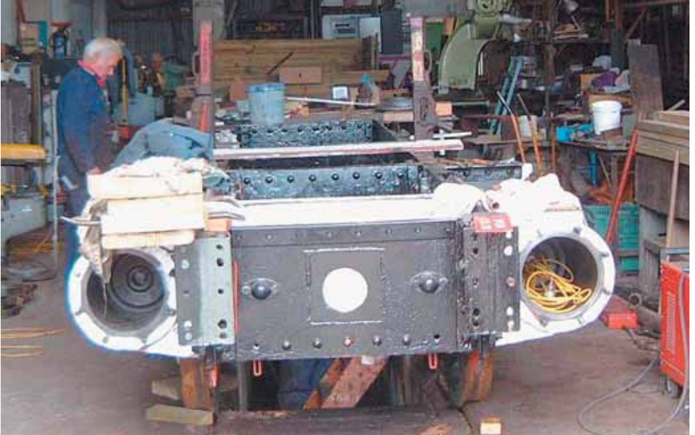
The rewarding sight of the frame resting on its axles at last.
