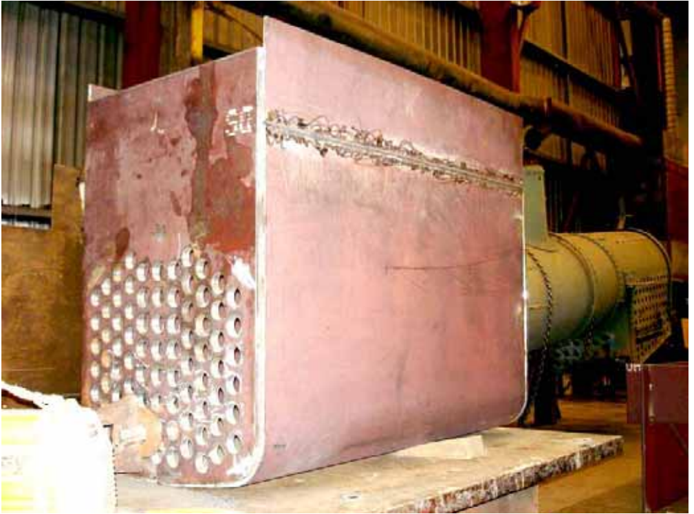
The new inner firebox shell, viewed from the tubeplate end.
