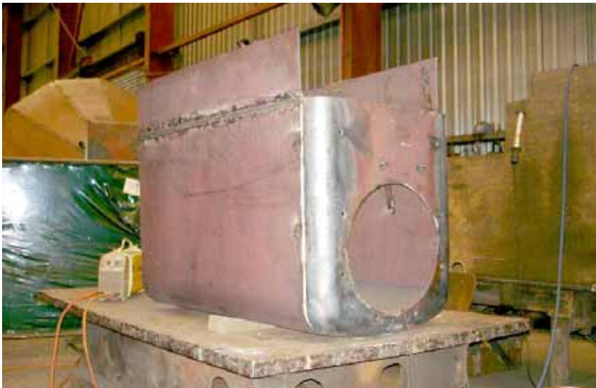
Upside down, we see the new inner firebox with the formed firehole plate welded into place.
