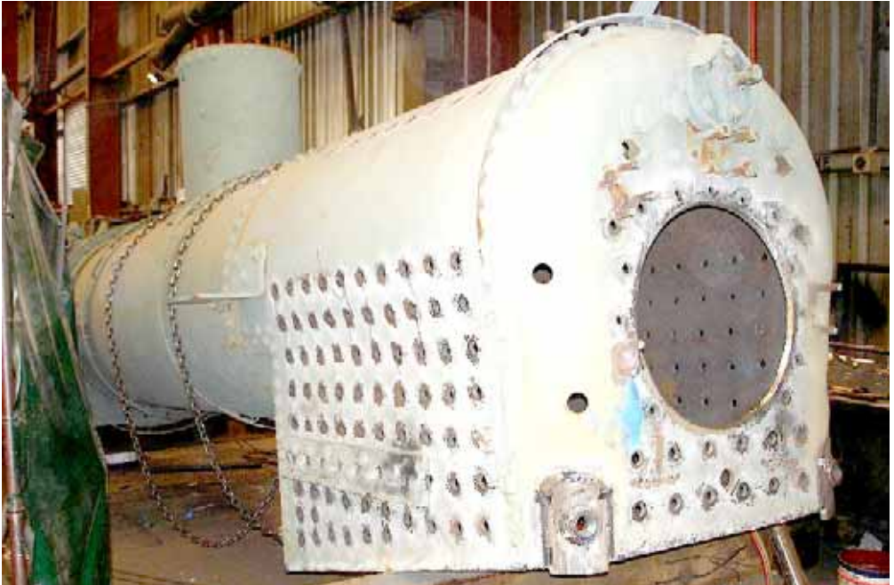
The shell with no innards. Sans inner firebox and tubes.
