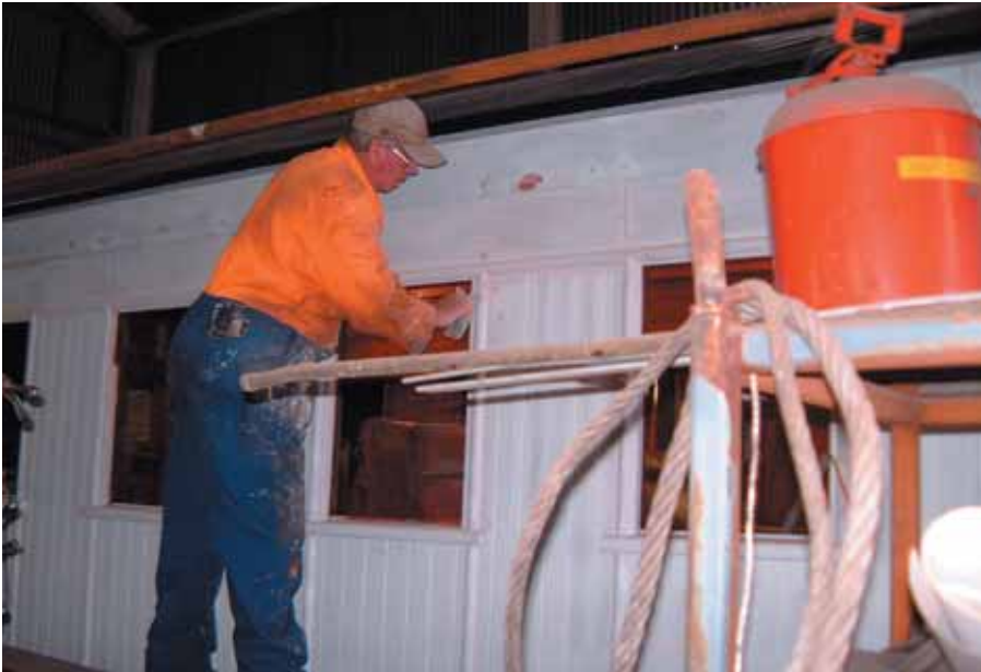
Max Anderson sands after puttying. On the other side, the window frames are painted and there are two coats of paint on the sides. Max has worked long and hard to get this far.
