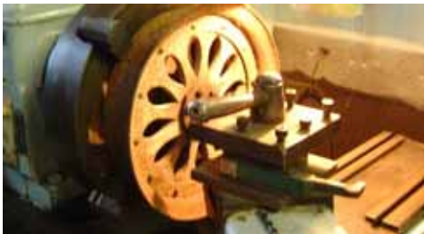
Boring a trolley wheel for a new trolley.
